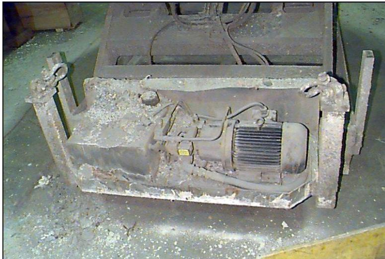
Figure 6 An example of an HPU whose cover was accidentally damaged during usage allowing mortar to accumulate inside. Had the HPU not been covered, the power unit may have required replacement instead of just a thorough cleaning.
