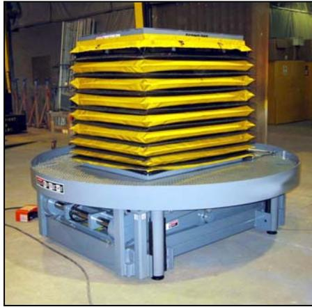
Figure 2 Example of collapsed ladle lift with secondary lift in raised position on top
