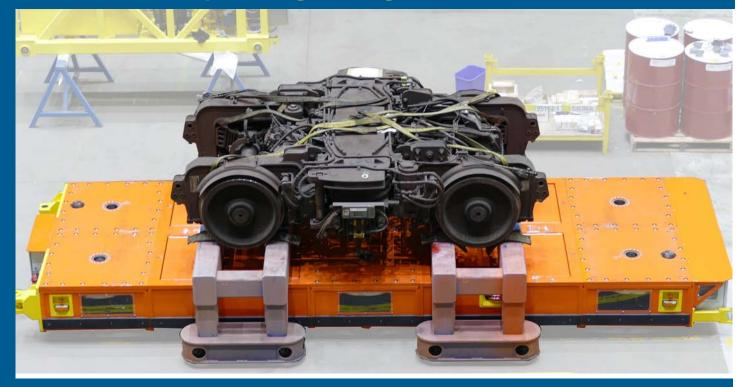
Handling Specialty's manually guided vehicles (MGVs) are designed to raise and traverse heavy loads and are robustly engineered for service in the rail/transportation industry. These highly flexible units can be fitted with specialized guidance sensors and advanced controls to provide automatic guidance capabilities.
